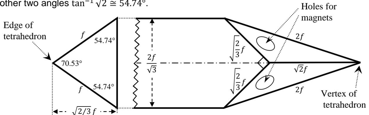
Figure 3. Cross-section of a strut, and bottom view of the end a strut.
