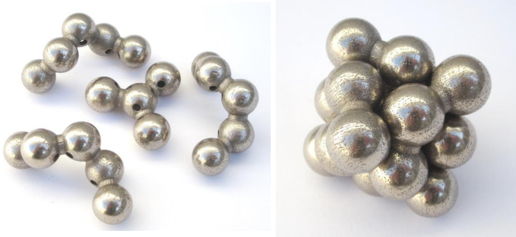
Figure 4. Screwy Octahedron CM, made from stainless steel using 3D printing [4].
