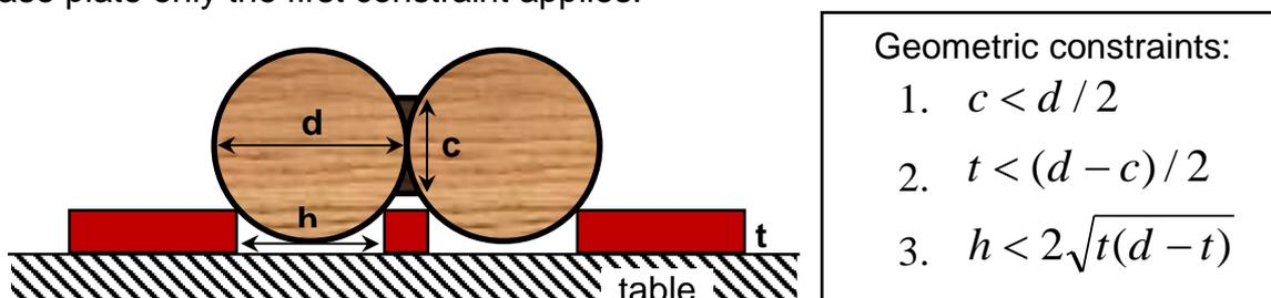
**Figure 4. Geometric constraints for ball pyramid puzzles and the base plate.**
