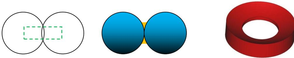
Figure 2. Two doweled balls pushed too close together, two balls glued together to form a “bi-sphere”, (much larger) a design for a connector to be 3D printed.
