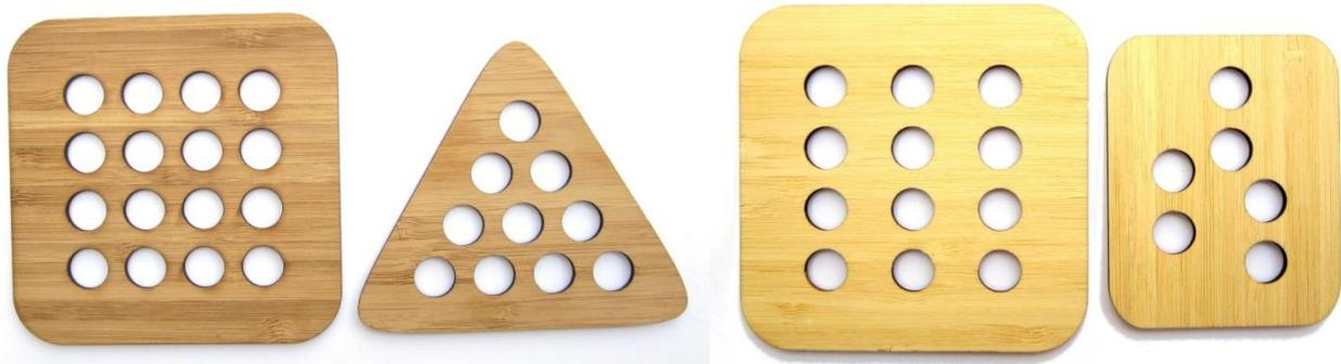
Figure 5. Some laser-cut base plates for 5/8" pieces. The rightmost plate is a jig for creating pieces with angles found in hexagonal sphere packing (see [10]).
